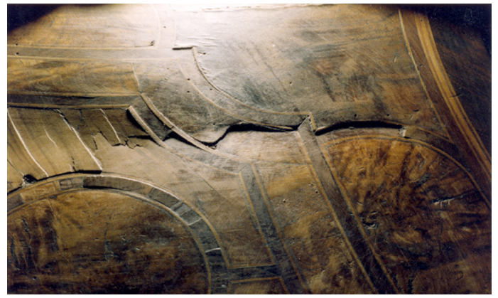
Figure 1 - Example of substrate shrinkage and movement creating marquetry surface damage.
