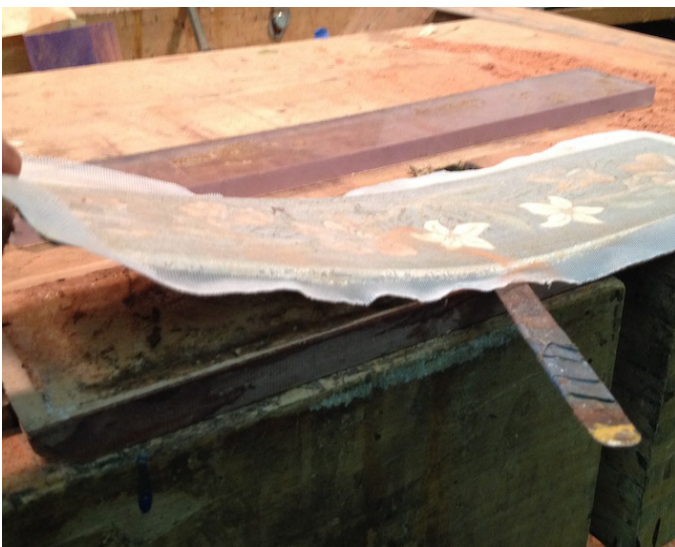
Figure 4: After application of tissue and neoprene glue, a heat gun and spatula is used to lift the marquetry surface in one piece.
