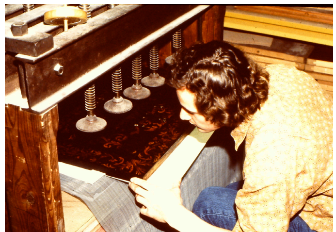
Figure 8: Thin sheet of Lexan placed directly on wet glue insures a flat reference surface. Shown is Nicolas Boucher, furniture Conservator at Museum of Decorative Arts, Paris.
