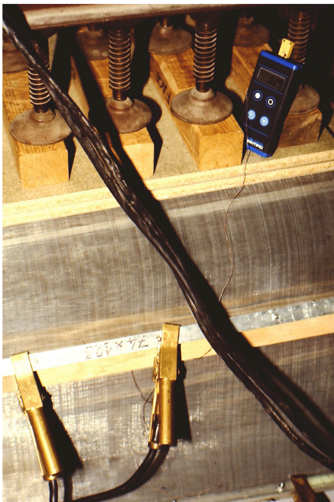
Figure 9: Marquetry panel, Lexan, card stock, heat sensor, and heating grill in press at 55° C.
